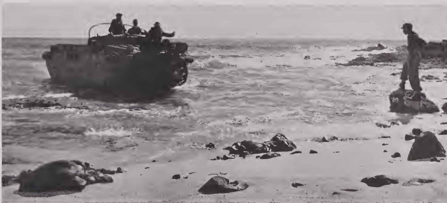
FIGURE 5. DUKW driver brings his vehicle out of coral reef on to boulder-studded beach during training course at Waimanalo. Instructor watches from beach as lookout on bow guides his driver.
